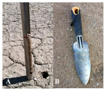
Fig. 1. A, soil sampling using augers with a mark of 6-inch depth, and B, small shovels with depth marks for soil sampling
